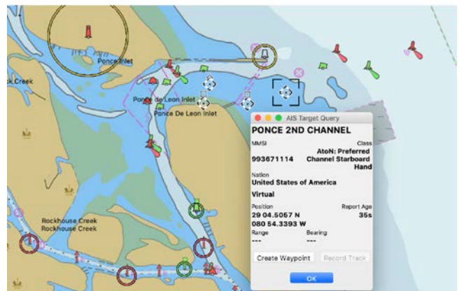
Figure 5. AIS display of real and fake virtual AtoNs in Ponce De Leon Inlet, south of Daytona Beach, Florida.
