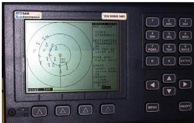
Figure 1. Basic AIS display and control unit provides a radar-like display of nearby targets. (Source: https://commons.wikimedia.org/wiki/File:Ais_dcu_bridge.jpg ) 1
