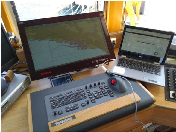
**Fig. 4** Testing setup for the vulnerability scanning of the shipboard ECDIS
