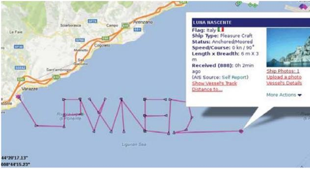
Figure 2: Example of spoofed ship following a programmed path.
